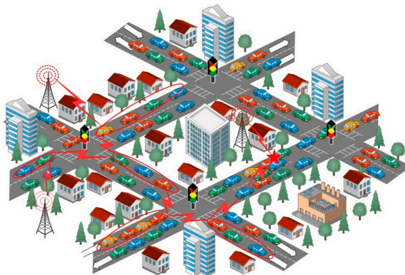
Figure 1. Vehicle-to-Vehicle (V2V) and Vehicle-to-Infrastructure (V2I) communication.
