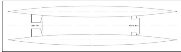
Figure 2 Position of fore fin and aft fin on hull
