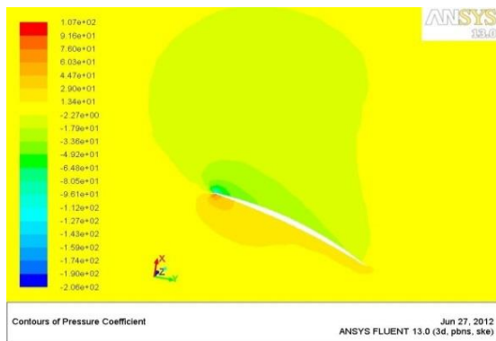
Figure 4 Contours of pressure coefficient on blade section
