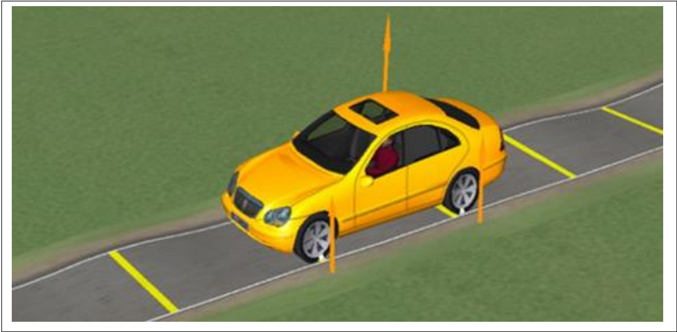
Figure 12 Virtual animation by CarSim for active suspension system with CCNF
