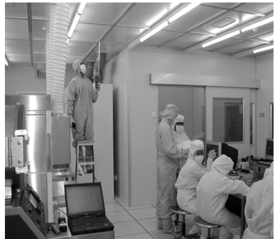
Figure 13. Airbone particle count test in progress.
