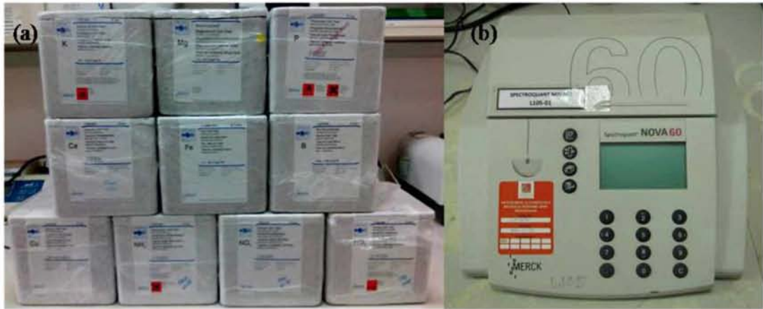
Figure A5 (a) Spectroquant® test kits and (b) Spectroquant® NOVA 60 analyzer used for macro- and micro-nutrients analysis. From left to right are the test kits for (first row) Potassium, Magnesium and Phosphorus; (second row) Calcium, Iron and Boron; (third row) Copper, ammonium, nitrate and nitrite.
