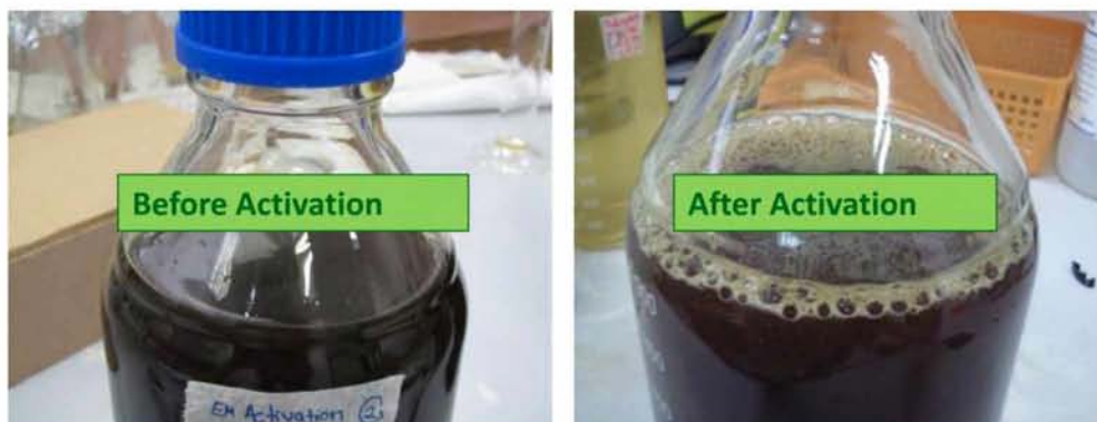
Figure A3 EM solutions before and after activation. Fully activated EM gave a lighter color and gas production can be observed along the one week activation process due to the microbial respiration.
