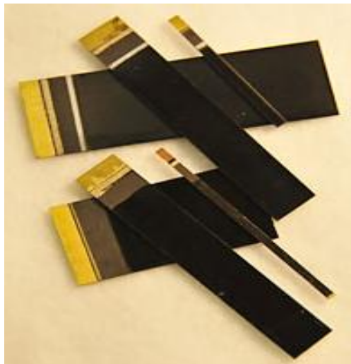
Figure 1.5 Strip actuator, which offers large stroke with limited blocking force.
