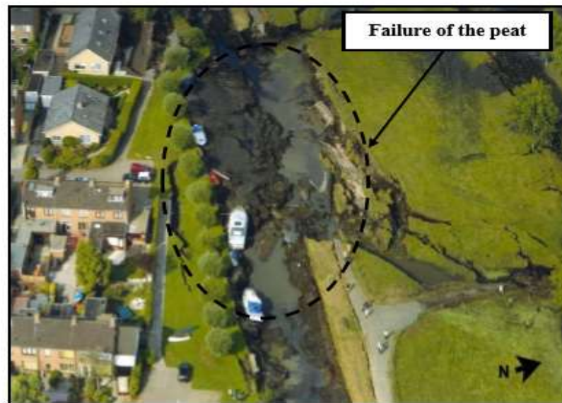
Figure 1.3 Failure of peat dyke due to drought in Netherlands
