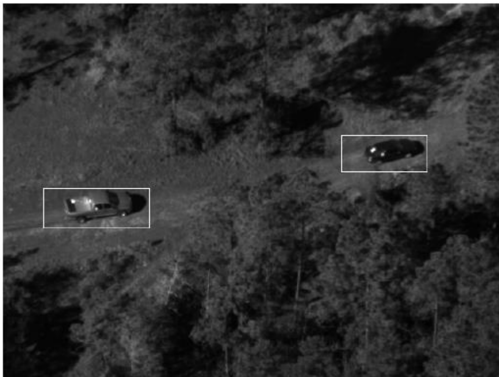
Figure 1.1 Moving object detection and locating from video captured by camera on UAV [1]
