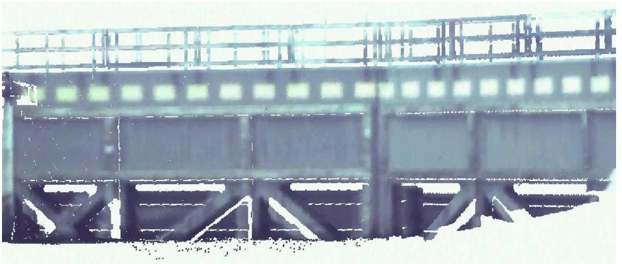
Figure 1.1 Point cloud representing points from the first epoch (Lindenberg and Pfeifer, 2005)
