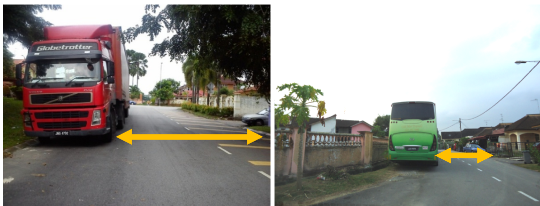
Figure 1-2: Heavy vehicle parking on lane and road shoulder has reduced the access width particularly for fire engines.
