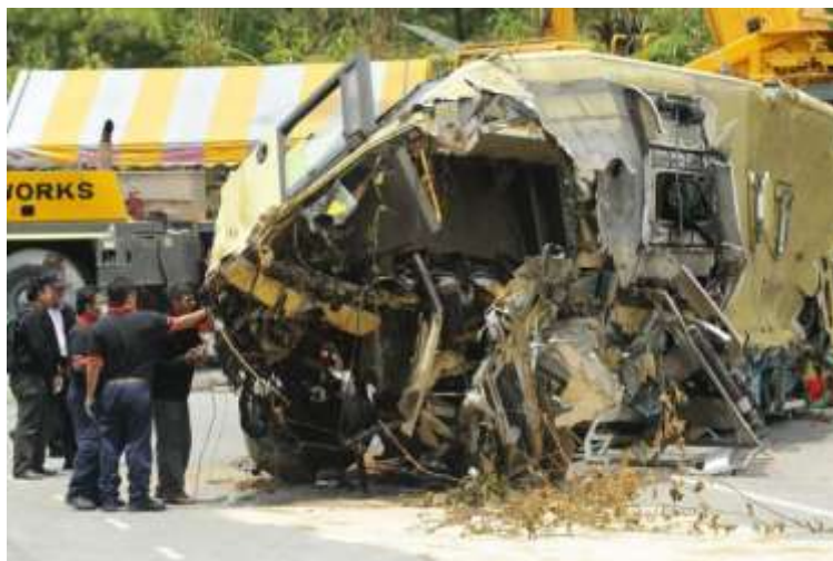
Figure 1.9 : Bus Superstructure after having a rollover accident in Genting Highlands
