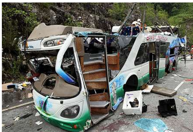
Figure 1.10 : Bus Superstructure after having a rollover accident in Cameron
