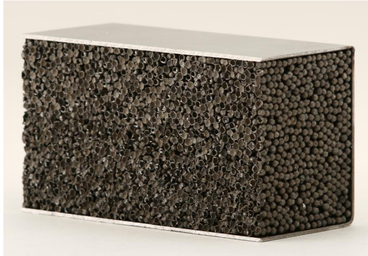
Figure 1.1 Aluminum profile filled with hollow sphere structures particles (Fraunhofer IFAM 2014)
