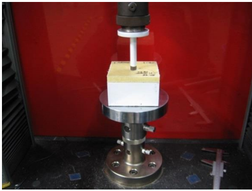
Figure 5 Indentation test of foam core composite sandwich panel
