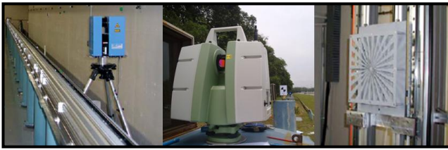
Figure 1 Facilities and devices required for component calibration [3, 5]
