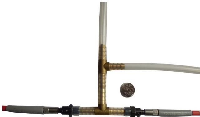
Figure 2 Gas cell of 5.6 cm optical path length that consists of two equal T brass gas connectors that are jointed together using silicone tubes. Gas cell is connected to collimating lens, optical fibers, ozone gas inlet and outlet. Size of gas cell is compared to Malaysian 10 cent coin
