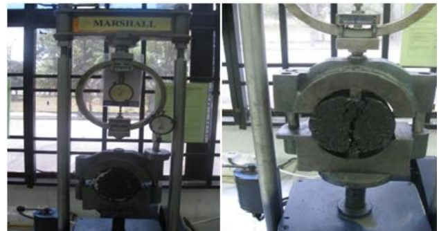
Figure 3 Indirect tensile strength test equipment used through the study
