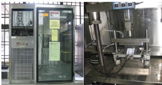
Figure 2 Universal testing machine (left) and arrangement sample for resilient modulus test (right)
