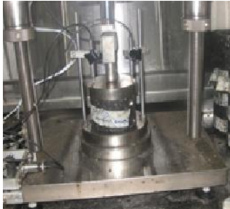
Figure 5 Dynamic creep test equipment used in this study
