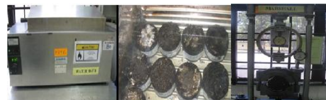
Figure 4 Stability test apparatus used this investigation
