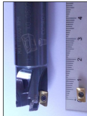
Figure 2 Tool holder and insert used for HSEM
