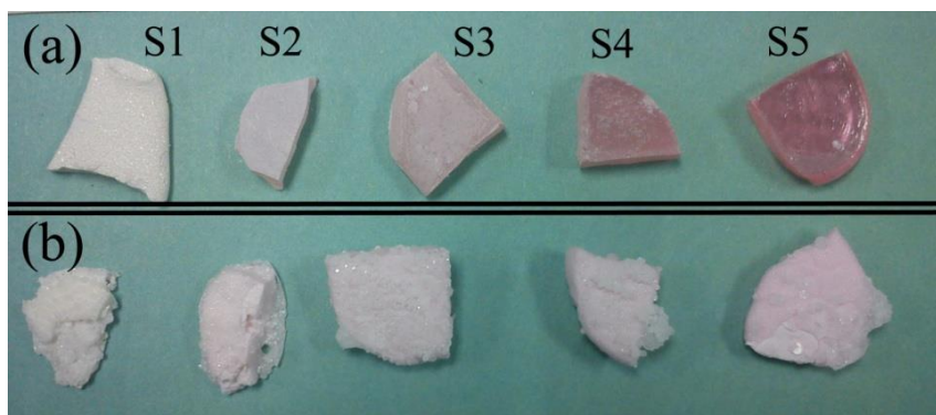
Fig.2. Increase of transparency of samples kept in water (a) and \text{NH}_4\text{OH} (b) after 4 days by addition of erbium content in zinc boro-tellurite glass.
