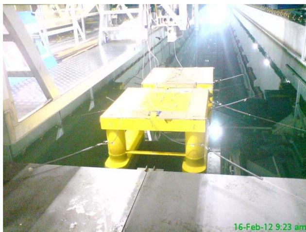
**Figure 8** TLP and Semi Submersible set up into towing tank
