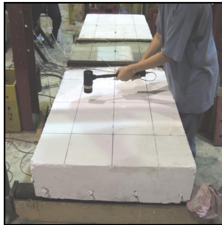
Figure 3 Conducting modal test on the prestressed concrete panel in the laboratory
