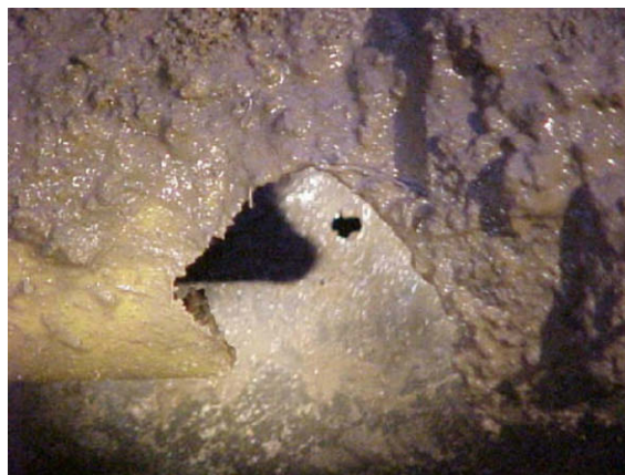
Fig. 7. In-situ PE pipe directly 'in the line of fire' of the API 5L X42 gas jet.
