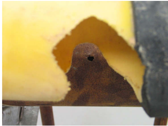
Fig. 8. Repositioned of API 5L X42 and PE pipe in lab (after excavation) truly match with Fig. 7.
