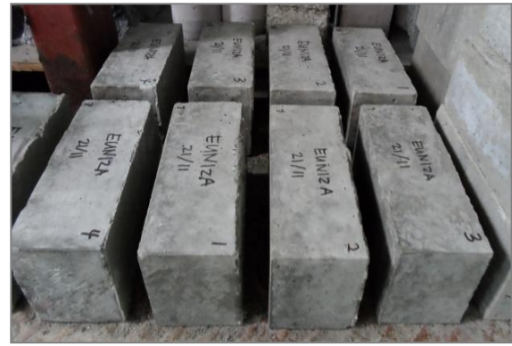
Figure 3 Air curing of concrete paving block
