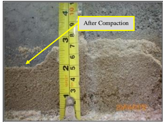
Figure 6 Settlement of concrete paving blocks after two cycles of compaction.
