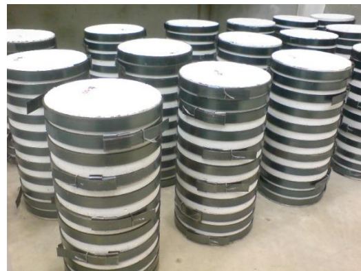
Figure 1 SSTT-confined high-strength concrete specimens
