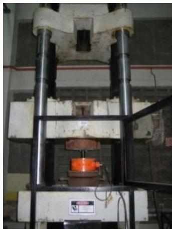
Figure 2 Diagram for (a) strain measuring equipment and (b) the loading device (TINIUS OLSEN Super “L” Universal Testing Machine)
