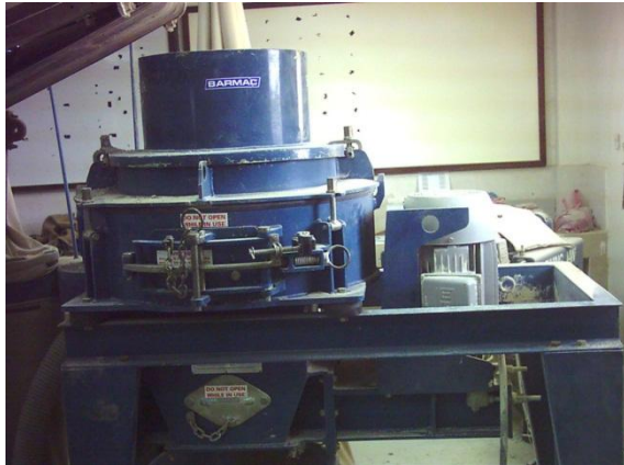
Figure 1 VSI crusher used to produce geometrically cubical aggregates
