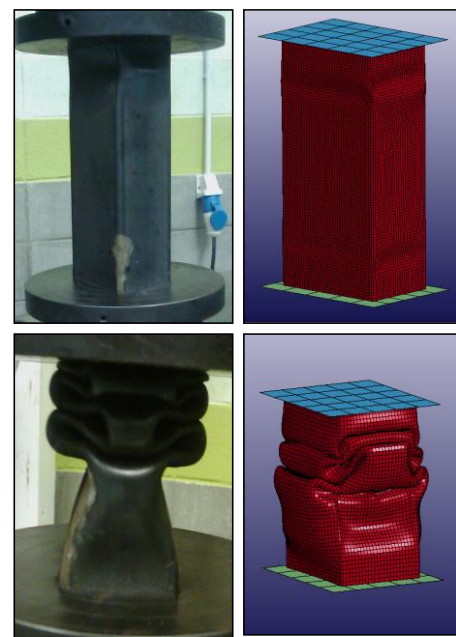
Figure 2 Deformation modes obtained from experimental and numerical results
