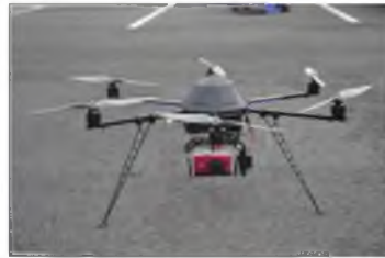
Figure 1. Hexacopter equipped with Canon PowerShot SX 230 HS.
