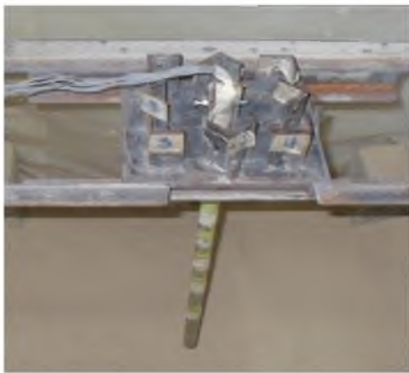
FIGURE 2: Pile and pile cap setup in soil box.
