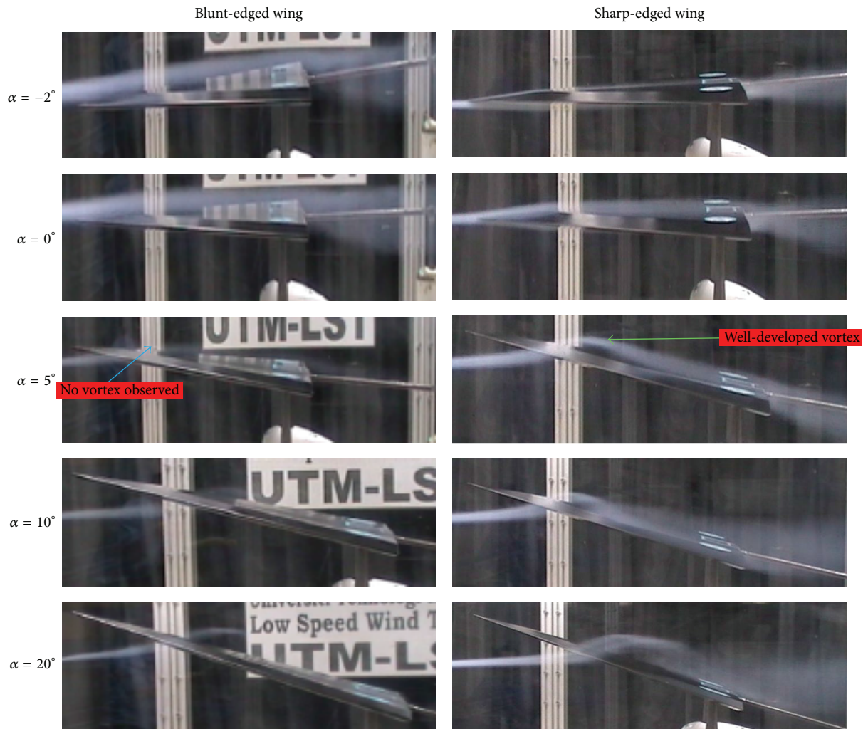
FIGURE 7: Table of smoke test at different angle of attack ( \alpha ) with each wing.
