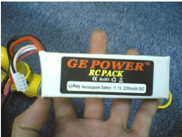
Figure 11 ROV 12 volts 220 mAh Lithium Polymer battery
