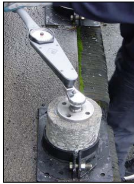
4a. Torque bond test device [55].
