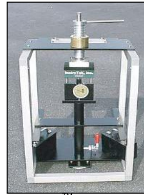
4b. ATacker™ test device [47].
