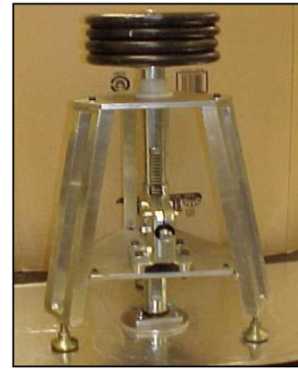
3c. UTEP pull-off test device [45].
