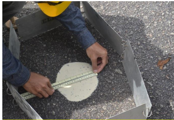
Figure 2 Sand patch test
