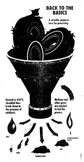
The Titan process breaks tires down. It operates at lower temperatures than other tire-melting systems, so it recovers high-quality products.
