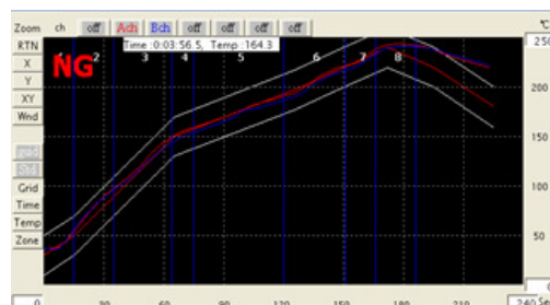
Figure 2. Reflow profile B with a fast post-reflow cooling rate
