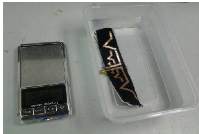
Figure 13. Antenna are tested under wet conditions.
