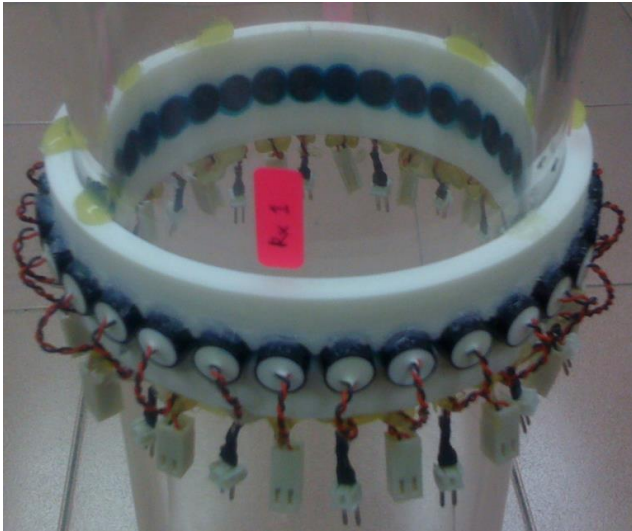
Figure 2 3D printed sensor fixture with installed ultrasonic sensors
