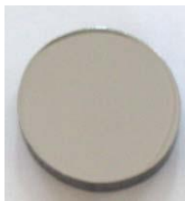
Figure 3 As-received carbon steel coupon
