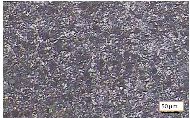
Figure 5 Optical micrograph ( \times 570 ) of uniform pitting on the carbon steel coupon exposed to iron bacteria inoculated medium for one month
