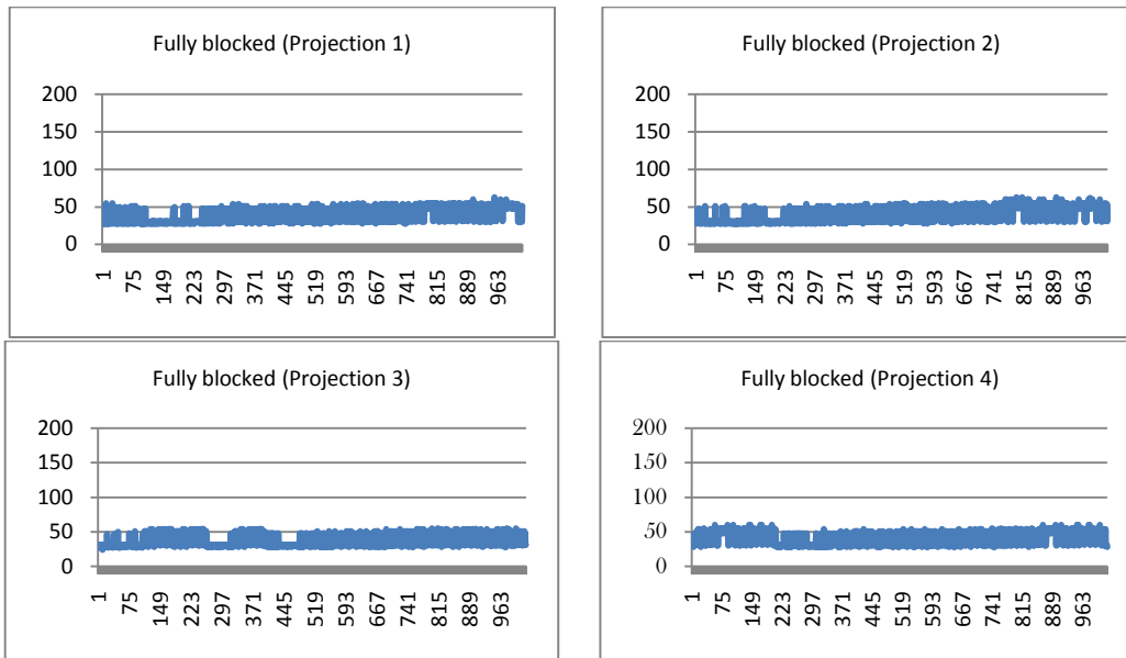
Figure 11 Result for fully blocked testing for four projections CMOS sensor
