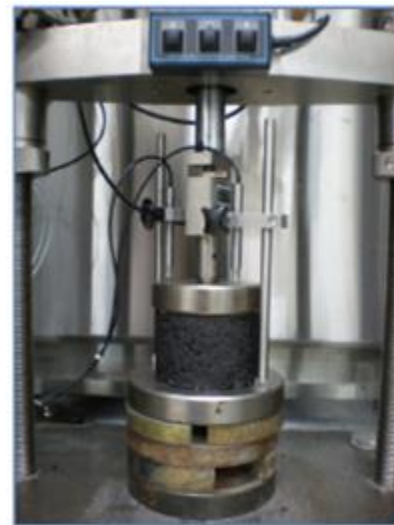
Figure 3 Fixing for creep test
