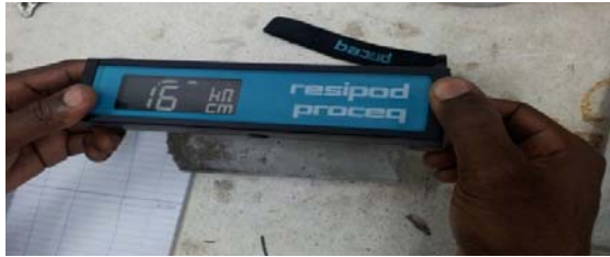
Figure-3. Concrete electrical resistivity measurement.
