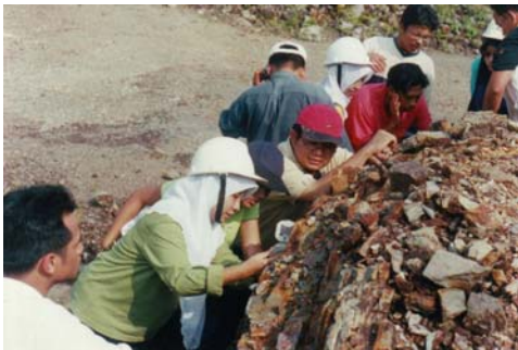
Figure 9: Measuring orientation of weakness planes in rock
