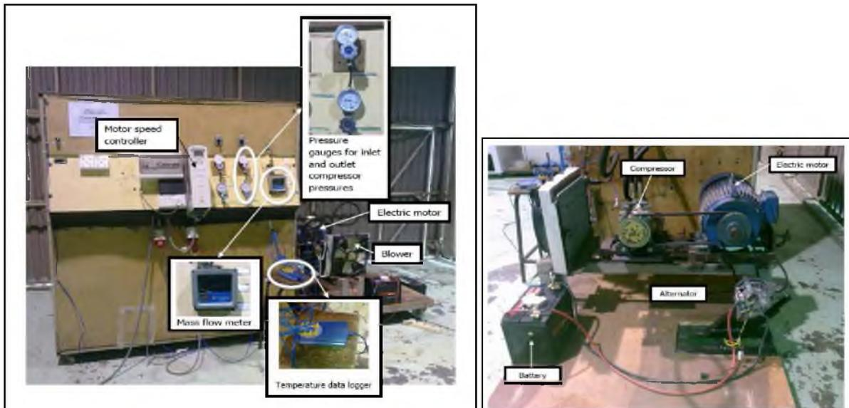
(b) Experimental test rig
