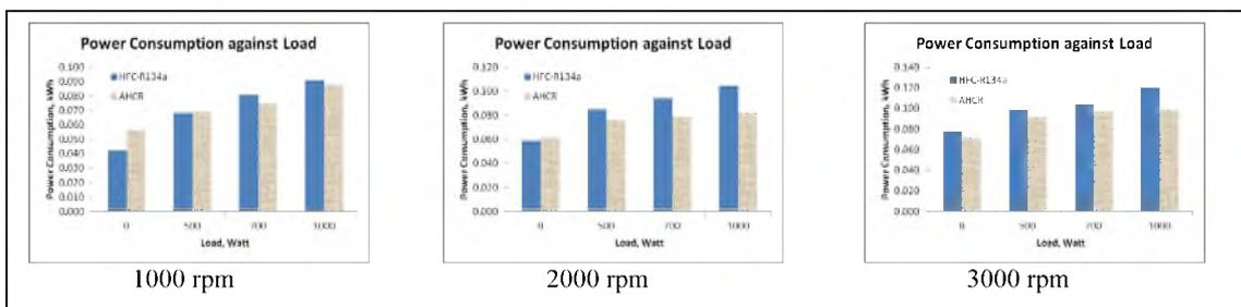
Fig. 3: Graph of power consumption against load (at compressor speed of 1000 – 3000 rpm).
