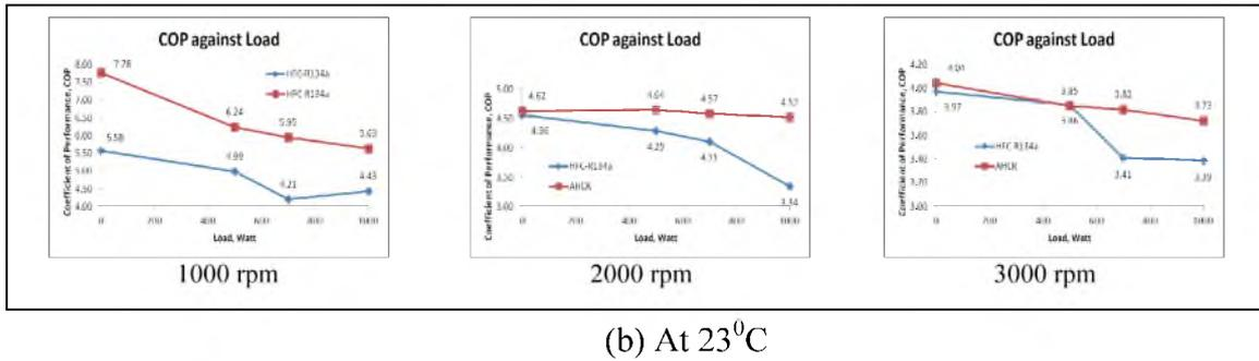
Fig. 2: Graph of COP against load (at compressor speed of 1000 – 3000 rpm).
