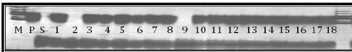
Fig. 1. Marker assay of F_1 plants of Shaheen Basmati \times Pokkali cross by amplifying the microsatellite locus RM263 on chromosome 5. Pokkali (P) and Shaheen Basmati (S) exhibited 170 bases and 160 bases, respectively. True hybrid seedlings exhibited both bands (170bp and 160bp), whereas self seedlings (2 and 9) showed a single band (160bp).
