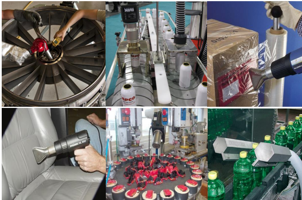
Figure 1.0 Various applications of a hot air blower in industrial
