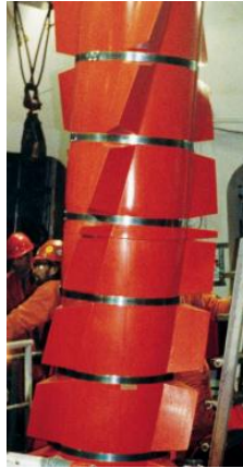
Figure 1.1: Passive type Vortex induced vibration suppression strake by Trelleborg CRP.
