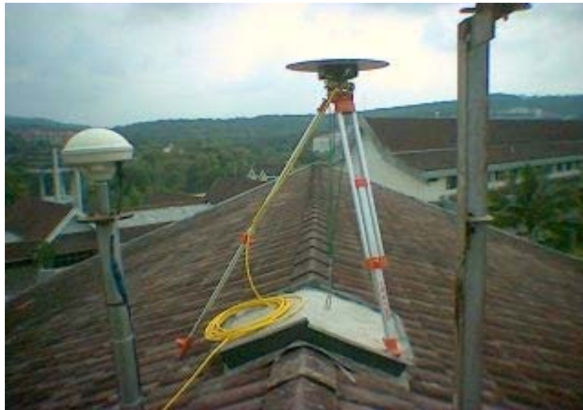
Figure 2: FKSG Trimble Reference Station
