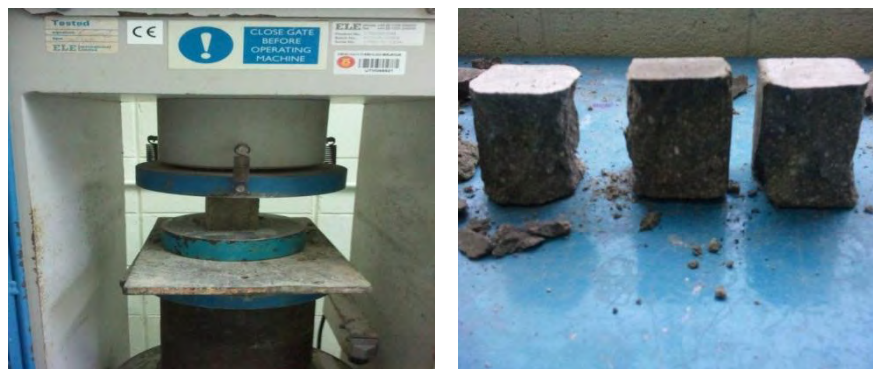
Figure 3.8: Compressive Strength Test
