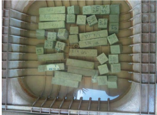
Figure 3.7: Curing of mortar in the water
