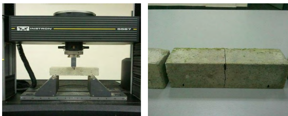
Figure 3.9: Flexural Strength Test
