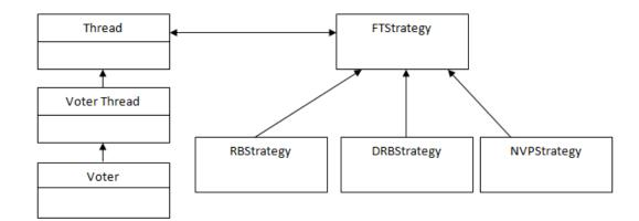
Figure 1.2 Fault tolerance framework (Afonso and Silva, 2008)
