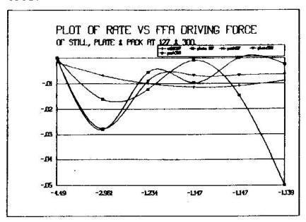
Conversely, the packed column exhibit a distinct Cubic order of equation with a higher stripping rate and over a wider operating condition but has instability in moving from one regime to another. Responses to disturbances are faster and more sensitive unless well controlled. Invariably this means better process control is needed especially on the distribution of liquid and vapor.
